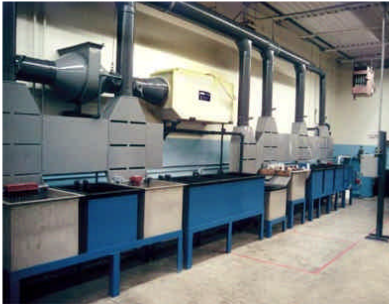
FIGURE 3. MCP Standard Electropolishing System consisting of twelve processing stations, 60-gallons nominal capacity, with SCR power supply equipped for precision polishing, ventilating system, atmospheric evaporator, mist eliminator, and remote operator control panel. The line produces extremely high quality technical finishes for clean gas distribution systems.
