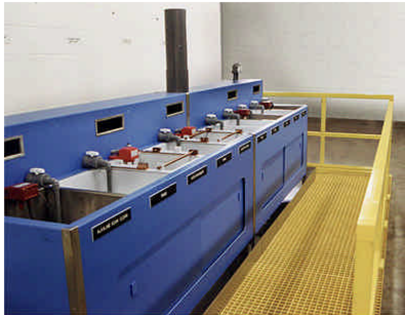
FIGURE 2A. Typical console electropolishing system designed for prototype development at a major manufacturing company. This installation includes 2 precleaning and post-treatment modules.
