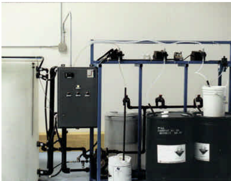
FIGURE 5B. Semi-automated batch waste treatment unit neutralizes up to 2000 gallons of rinse water per shift. The system can be upgraded for automatic operation by modification of the computer control. An optional filter press can be added to minimize operator supervision and to maximize throughput of waste water.
