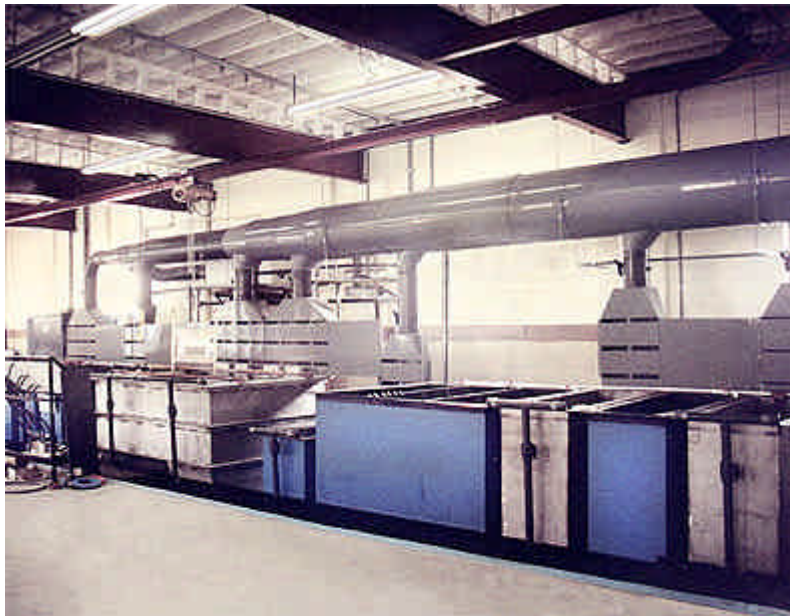
FIGURE 7A. This twelve-station line features a 1500-gallon electropolishing tank with a 6000-ampere power supply. The system is designed for handling large volumes of flat sheets for food manufacturing equipment.
